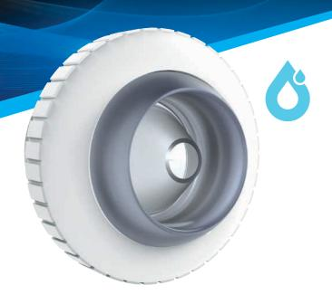
The patented dynamic eyeball at the center of the iBoosTPRO can vary it's opening; so as the pump speed reduces, the opening constricts to maintain water velocity.
